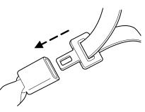
2. To unfasten, push the release button and remove the tongue from the buckle.
